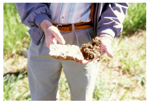
Development of soil crust reduces infiltration, causing more runoff and erosion.
